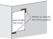
Once the mirror position is determined, use a marker like tape to indicate the position. (The illustration shows F15-EN as an example, which is a F33-EN horizontal type.)
