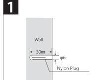
(1) Drill four holes 6 mm in diameter and 30 mm in length with a drill for concrete.
