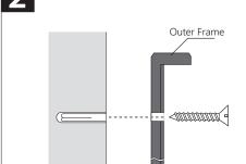
Screw the outer frame to the four plugs.
