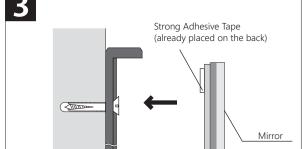
Remove the release paper from the strong adhesive tape and put the mirror into the outer frame.
